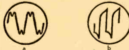
Fig. 3—Amplitude and harmonic distortion.
